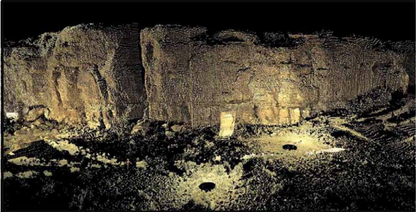
Figure 1. Overview of the model created from the mid-range laser scans of the landscape with the Leica Geosystems C10 ScanStation.
