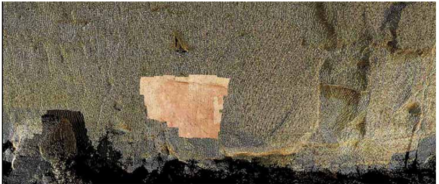
Figure 2. Zoom in view of model showing the Leica Geosystems ScanStation C10 aligned with the high resolution scans from the Breuckmann SmartScan 3D-HE .
